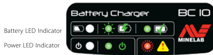
Figure 37 – BC 10 Front Panel
