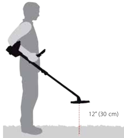
Figure 17 – Correct detector position for Noise Cancel
